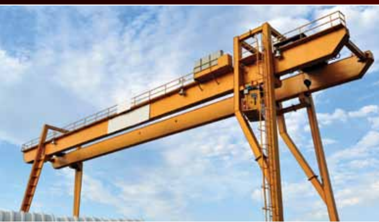
Double-leg Gantry with Cantilever
