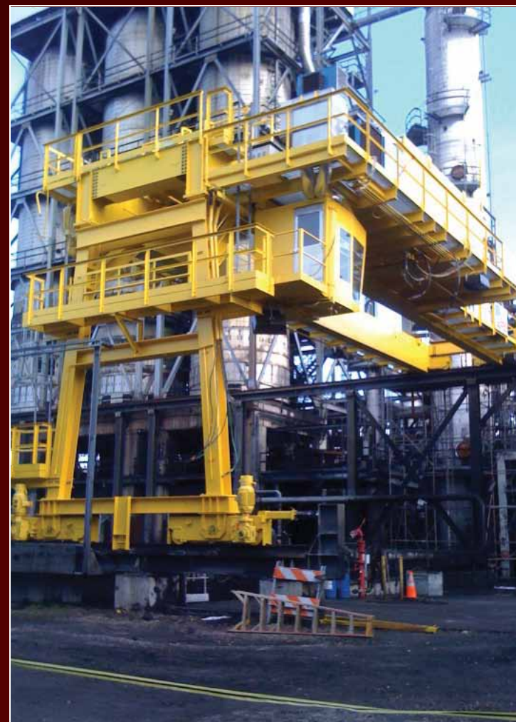
Semi Gantry Coker Crane
