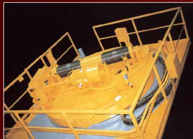
CMAA Class E, Polar Trolley for Billet Handling
