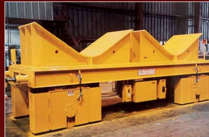
Transfer Car designed with shock absorbing wheel mounts to guard against damage to coils
