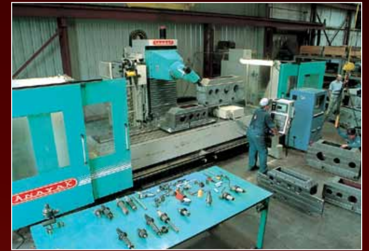
5 Axis CNC Machining Center for precision gearbox manufacturing
